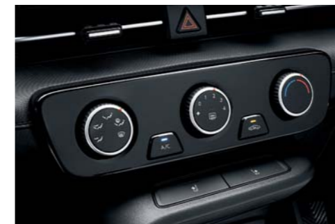
Manual air conditioning system
