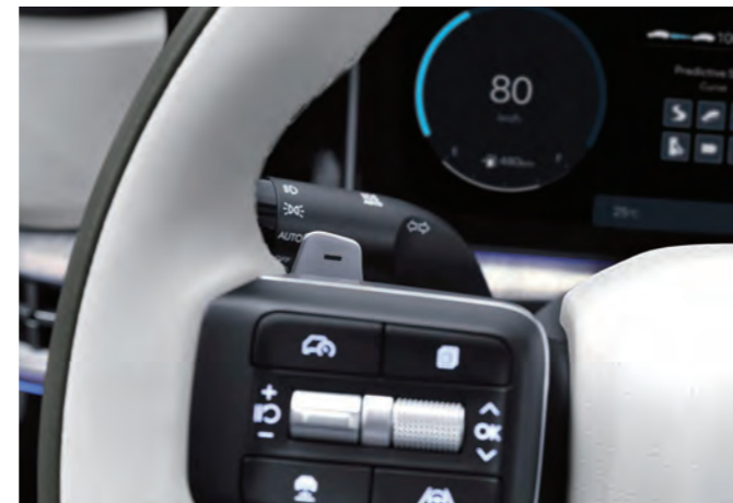
Hybrid Exclusive Features Paddle Shift-Regenerative Braking Mode
