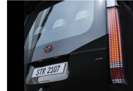
Parametric pixel lights (LED rear combination lamp)
